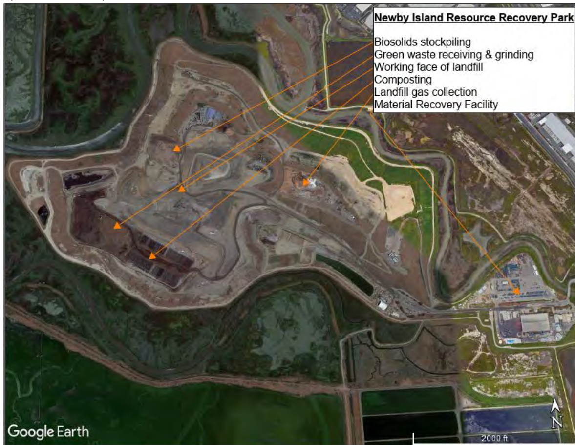
Figure 1-3. Newby Island Resource Recovery Park Facility Map, Milpitas, California (source: Google Earth)
