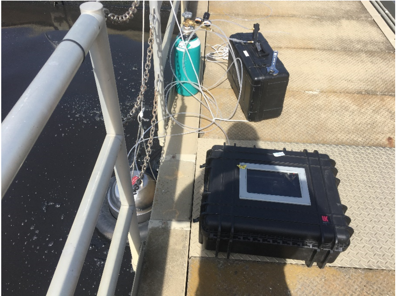
Figure E-8. Vacuum chamber for bag sample collection at RWF bioreactors
