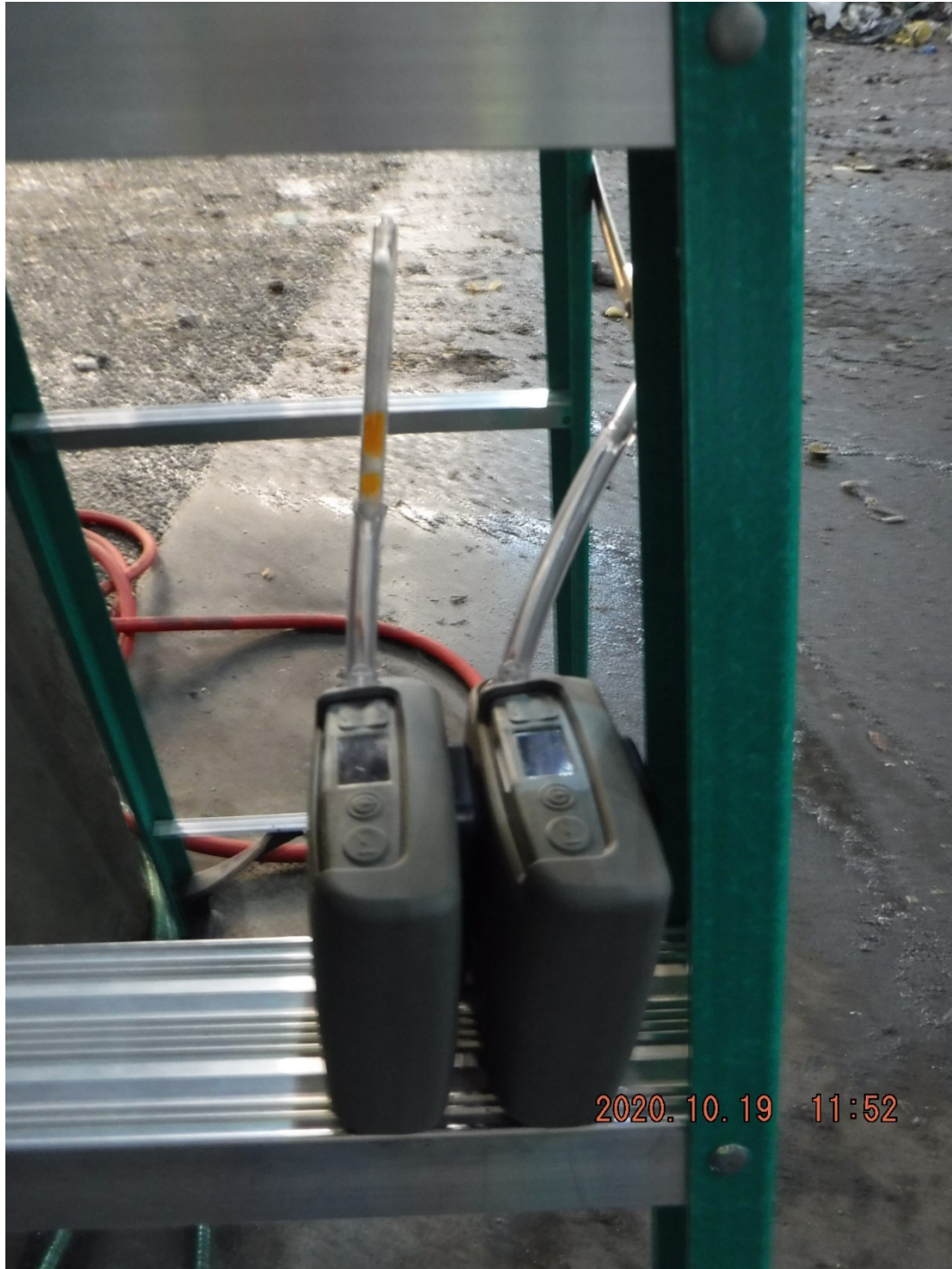
Figure E-3. Sorption tube placement at ZWED interior
