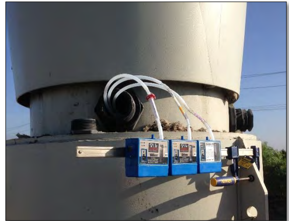
Figure 3-2. Sorbent Tubes and Sampling Pumps
