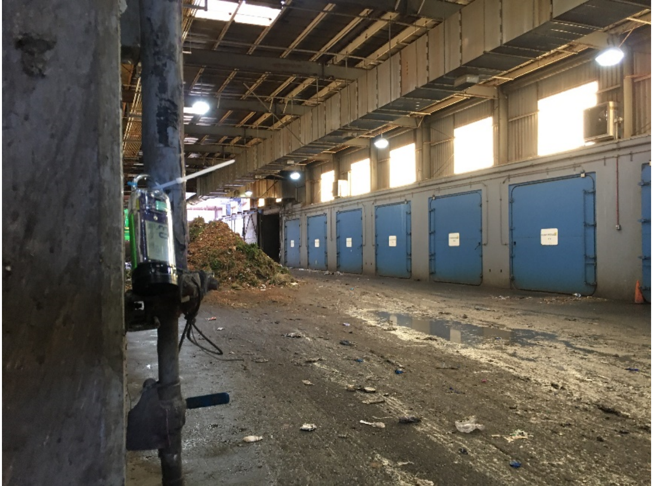
Figure E-15. Odor log unit deployed within ZWED interior space
