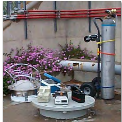
Figure 3-1. EPA Flux Chamber with Sampling Equipment
