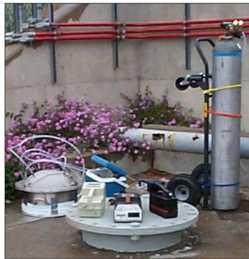
Figure 3-1. EPA Flux Chamber with Sampling Equipment
