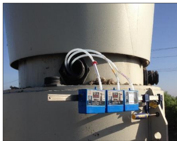
Figure 3-2. Sorbent Tubes and Sampling Pumps
