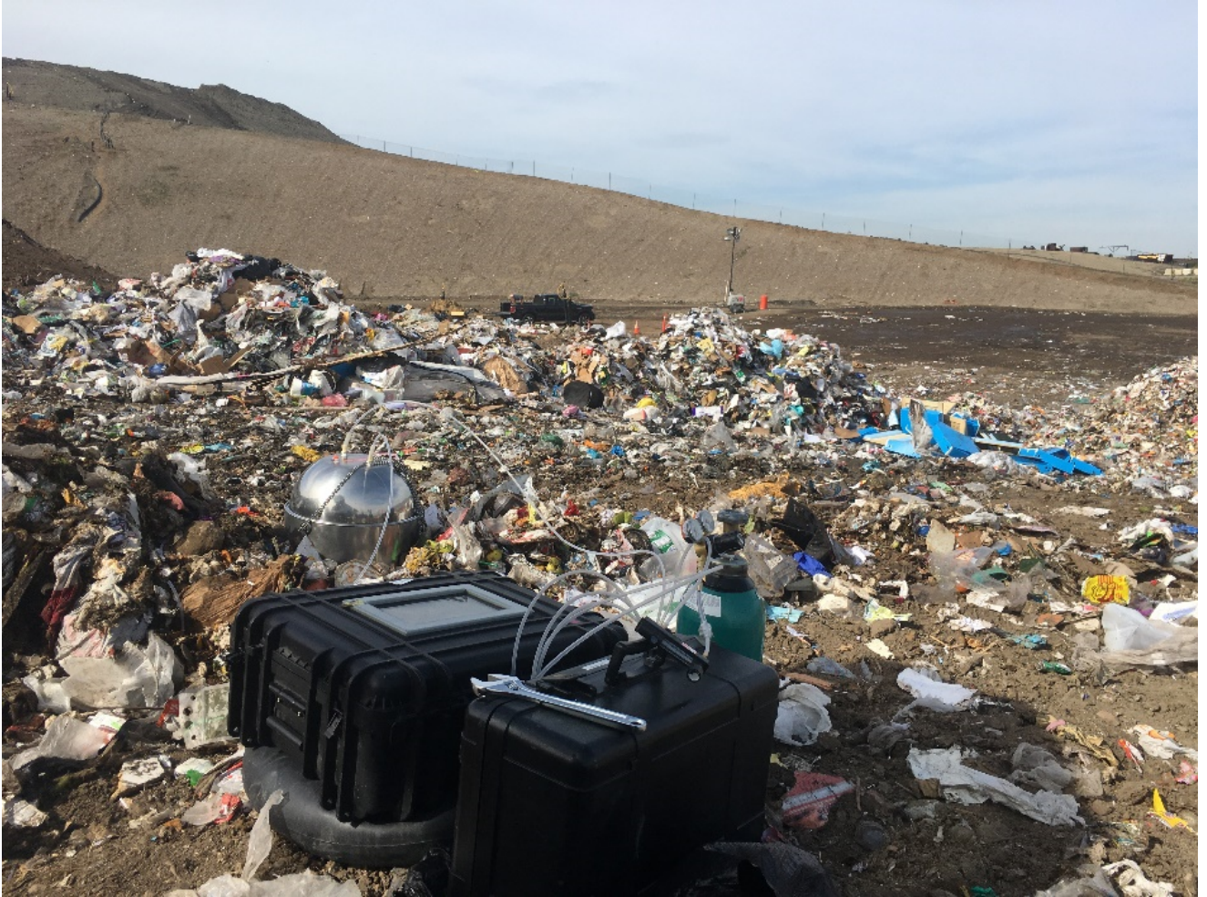
Figure E-10. Sorption tube collection with flux chamber at NIRRP working face
