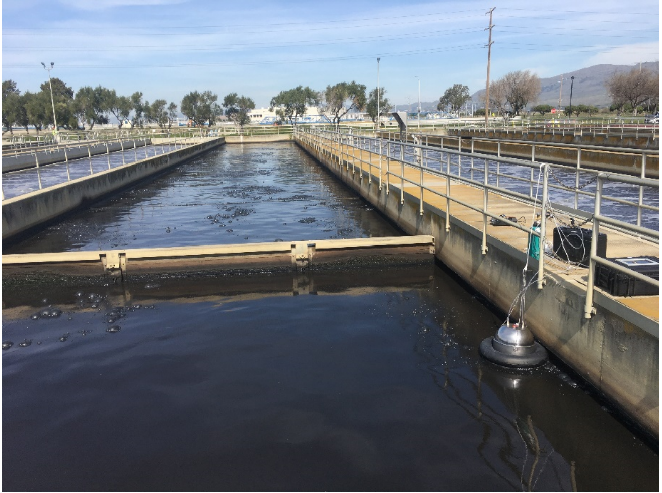
Figure E-9. Flux hood deployed on surface of RWF bioreactors
