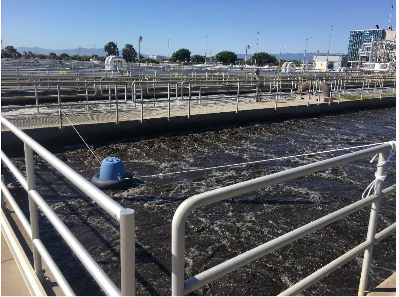
Figure E-14. Odor log with Mr. Floaty deployed on surface of RWF bioreactor
