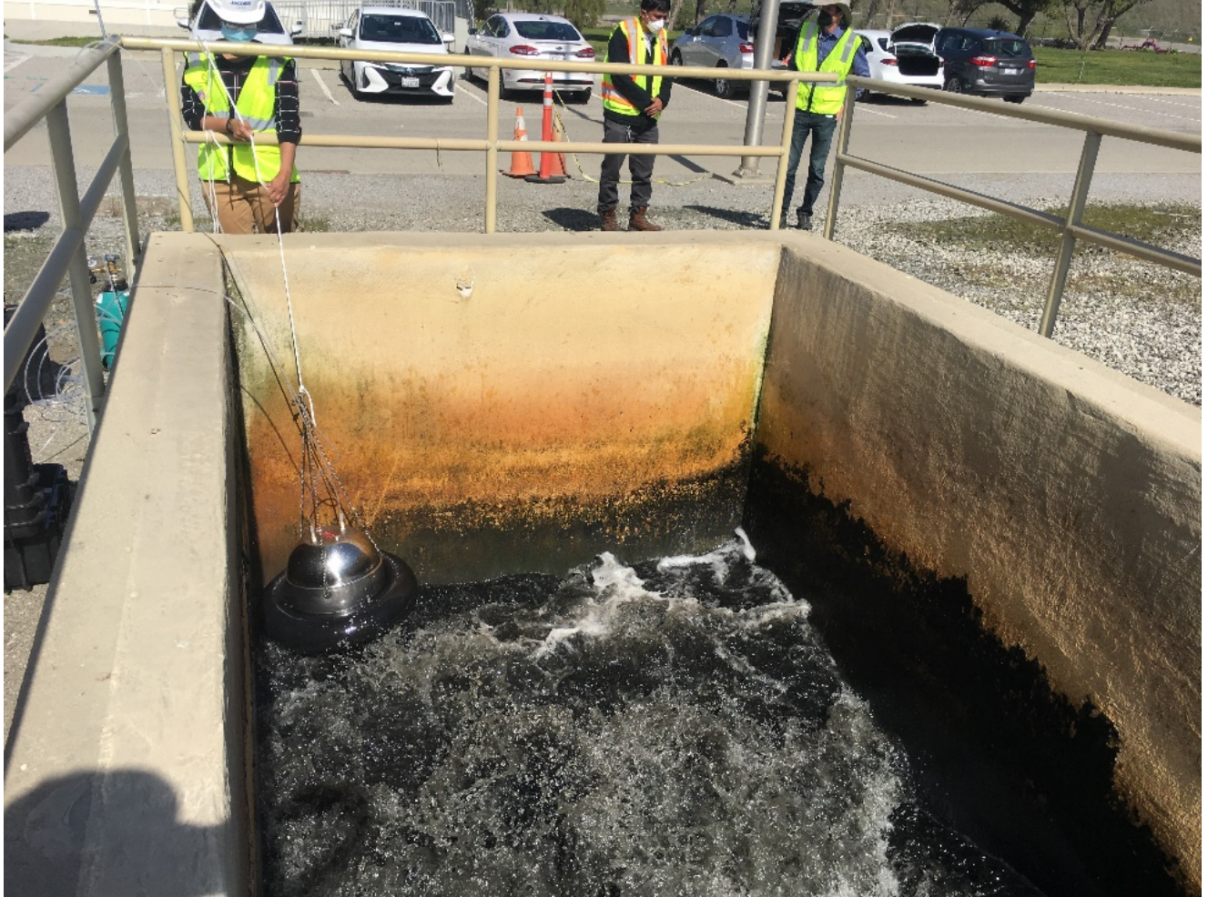
Figure E-11. Flux chamber deployed on surface of primary influent channel at RWF
