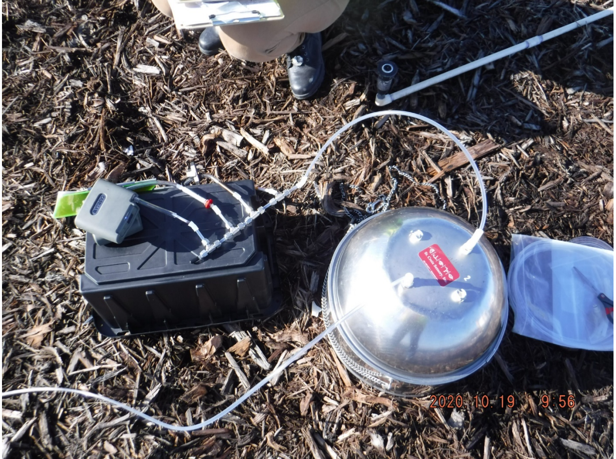
Figure E-2. Sorption tube assembly with flux hood on biofilter surface at ZWED
