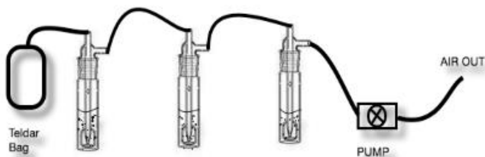
Figure 3-4. Set-up of Indole and Skatole Extraction System
