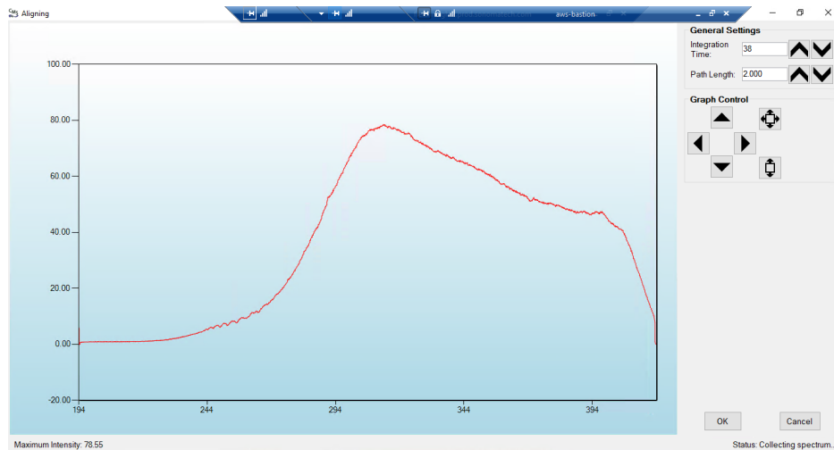
Figure 3. Screenshot for Align mode. The integration time can be entered in the upper right of the screen. In this particular screenshot, the integration time is 38 ms.
