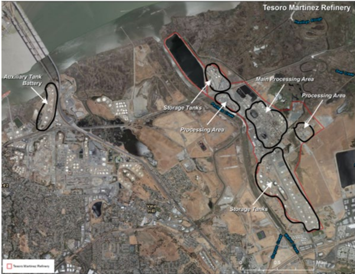
Figure 4. Layout of the Martinez Facility.
