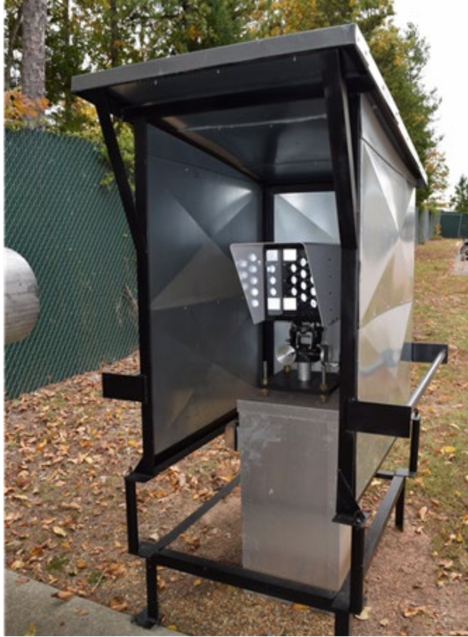
Figure 13. A UV-DOAS retroreflector.
