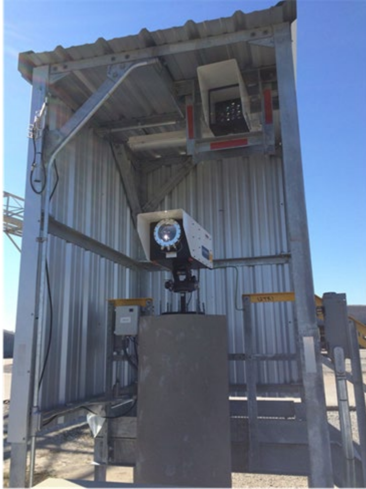
Figure 12. A UV-DOAS analyzer.
