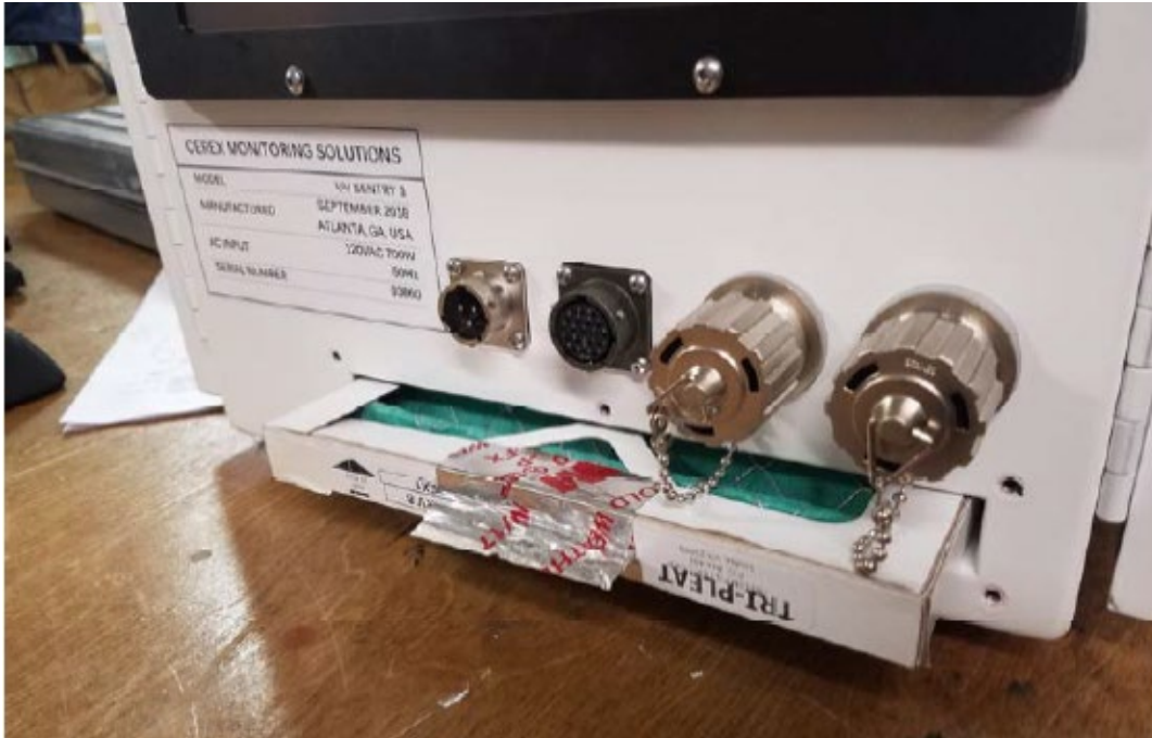
Figure 6. Filter access plate removed and filter partially removed.
