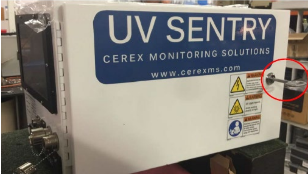
Figure 9. Opening the source access panel.
