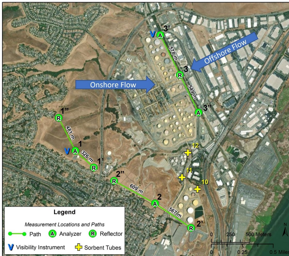
Figure 2. Open-path monitoring network for Valero’s Benicia Refinery. Each primary path is numbered and contains segments that are labeled with the path number and a prime (') or double prime (") symbol. Yellow "+" symbols indicate the location of point monitoring by sorbent tubes. Main wind flow directions are also shown.
