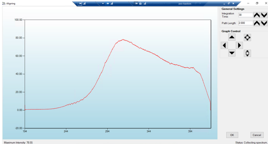
Figure A-3. Screenshot for Align mode. The integration time can be entered in the upper right of the screen. In this particular screenshot, the integration time is 38 ms.
