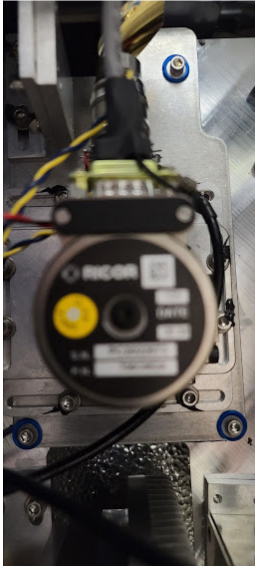
Figure B-6. Image showing baseplate and screws with rubber grommets.
