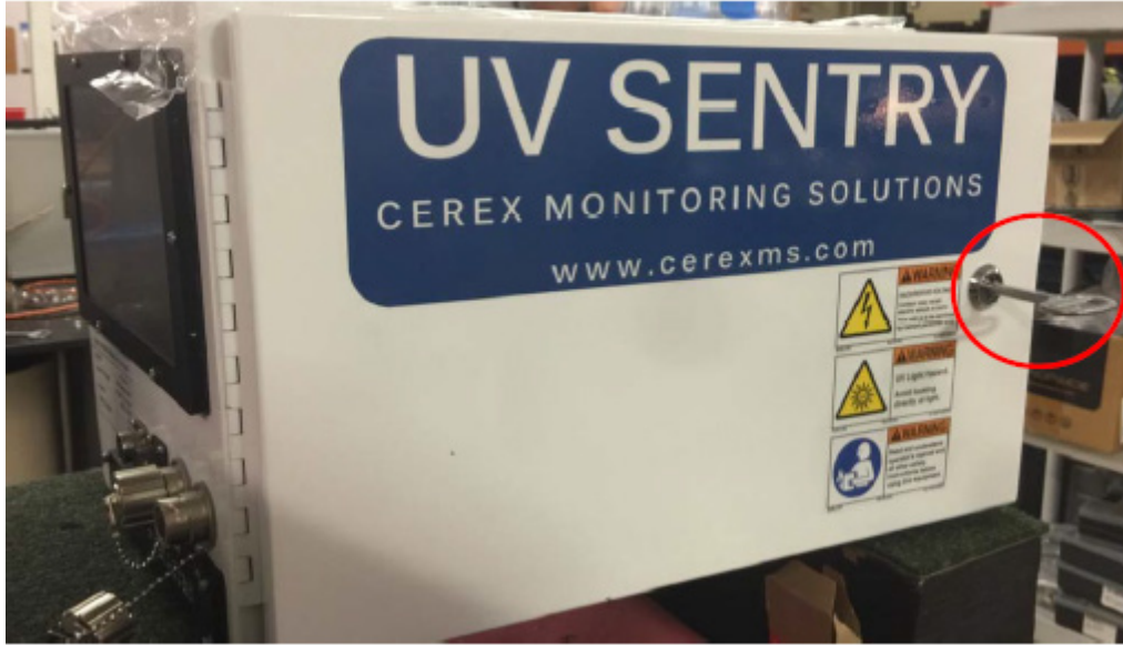
Figure A-9. Opening the source access panel.
