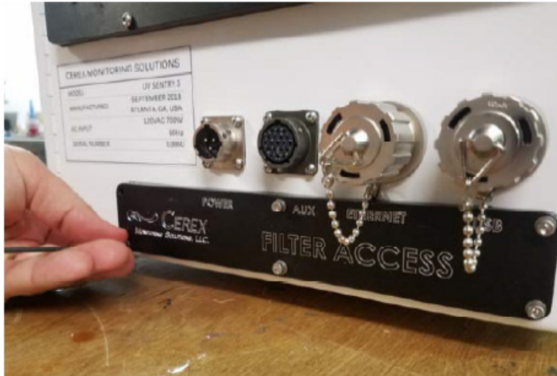
Figure A-5. Location of filter access plate.
