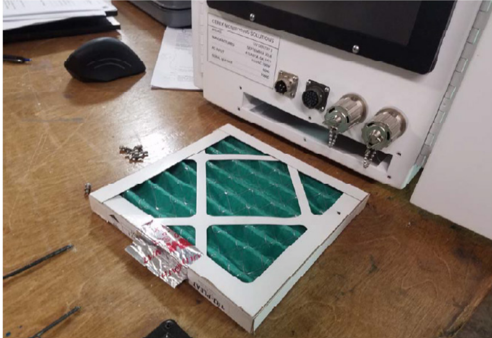
Figure A-7. Filter completely removed.
