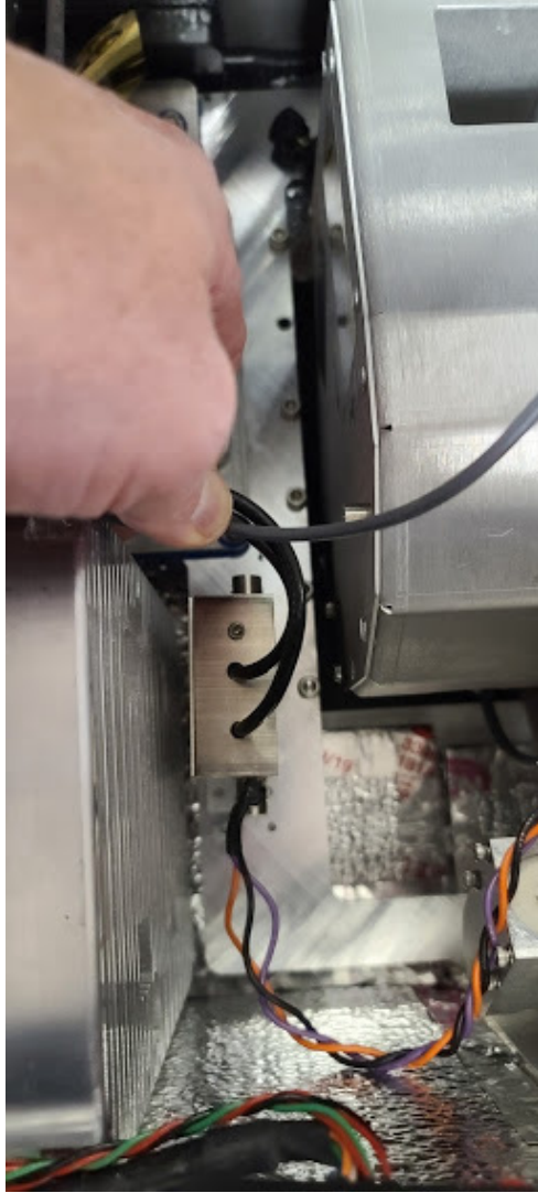
Figure B-7. Preamp assembly (with orange, black and purple wires) between the heatsink (left) and interferometer (right).
