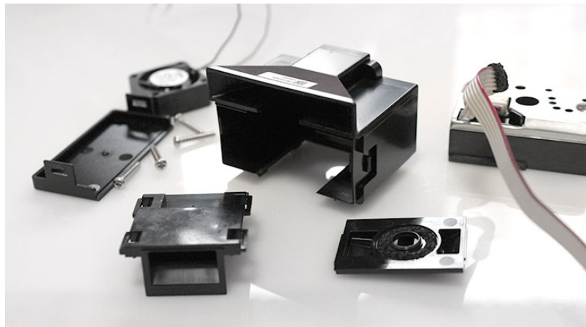
Figure 15: Sharp DN7C3JA001 with impactor, claimed to attenuate 98 % of response to d_p = 5.0\mu\text{m} (vs GP2Y1010AU0F).
